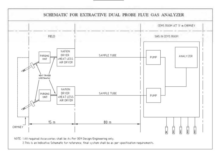
Note 12: Location of probe is at 48mts & analyzer is at '0'm of chimney. 15mts of HTL to be considered till Permapure Dryer in case of Extractive system. Permapure Dryer & Primary SHS shall be placed near probe at 48m elevation.
